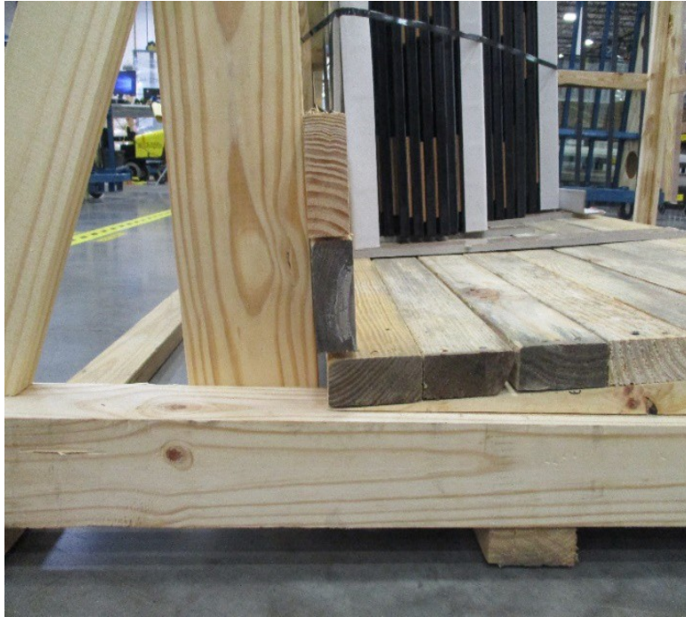
Figure 6: Back wall is designed with a slight angle to ensure units do not tip.
