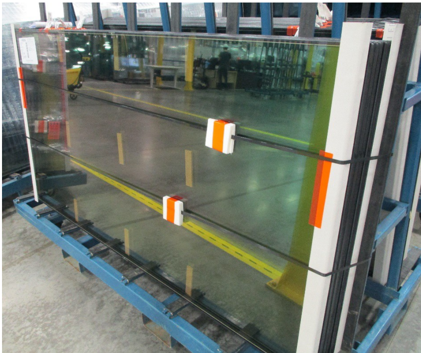
Figure 16: Units are secured to A-Frame and prepped to wrap.
