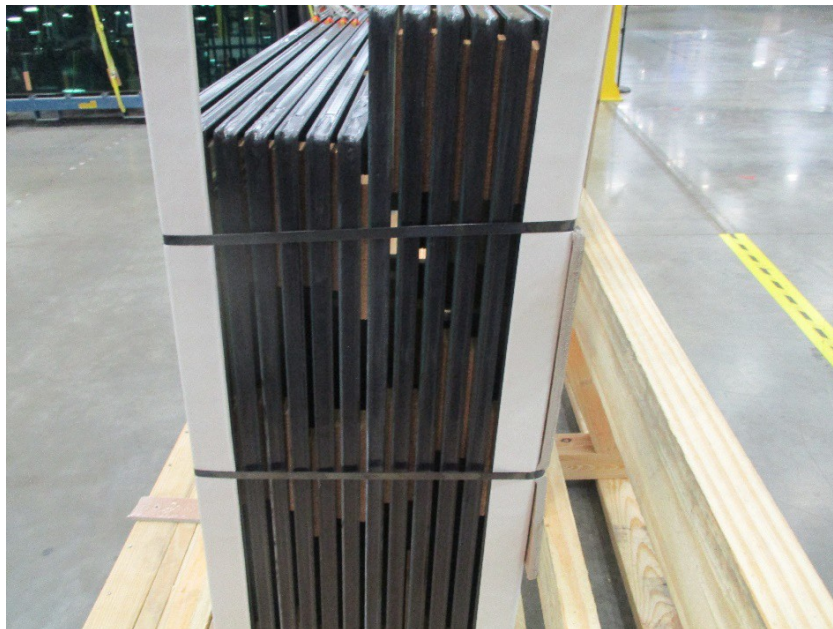
Figure 10: Plastic banding is placed on the outside of the crate to secure crate.
