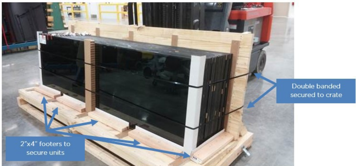
Figure 11: Units secured with 2 x 4 banding and angled cardboard. 2x4 boards placed to secure movement.
