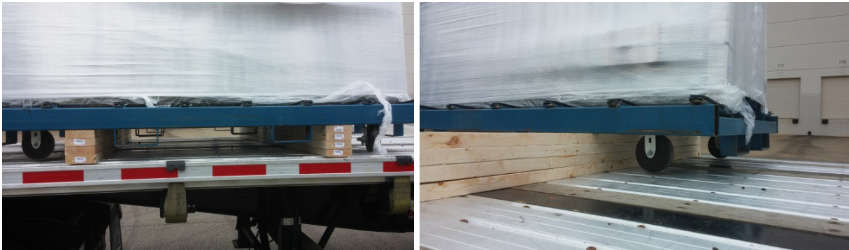
Figure 20: Frame is aligned neatly onto 8 2x4 boards.
