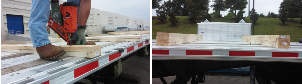
Figure 19: Nail 4 boards on each side to secure frames.
