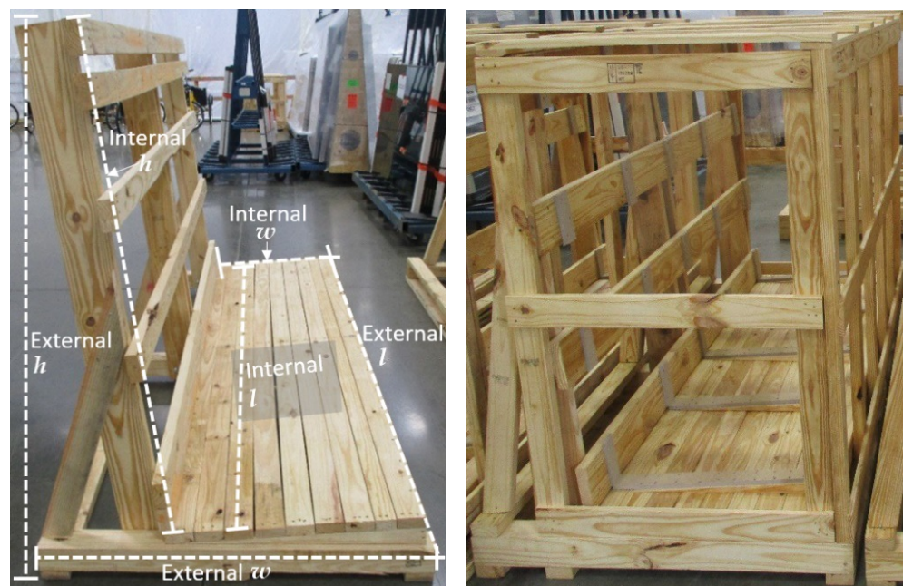
Figure 2b: Wooden Crate Types (Internal & External Dimensions).
