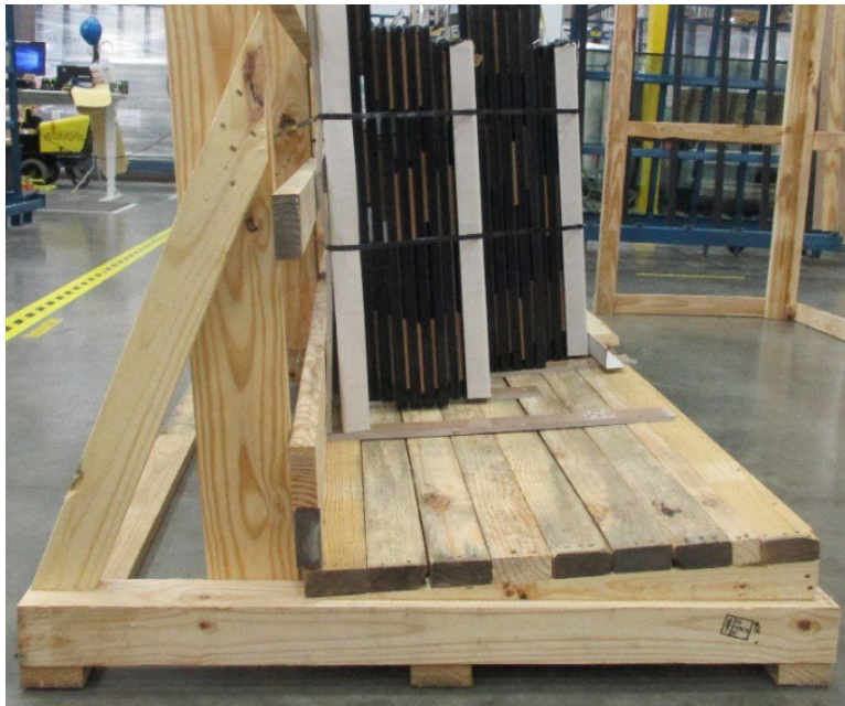
Figure 7: Large base to ensure crates do not tip.
