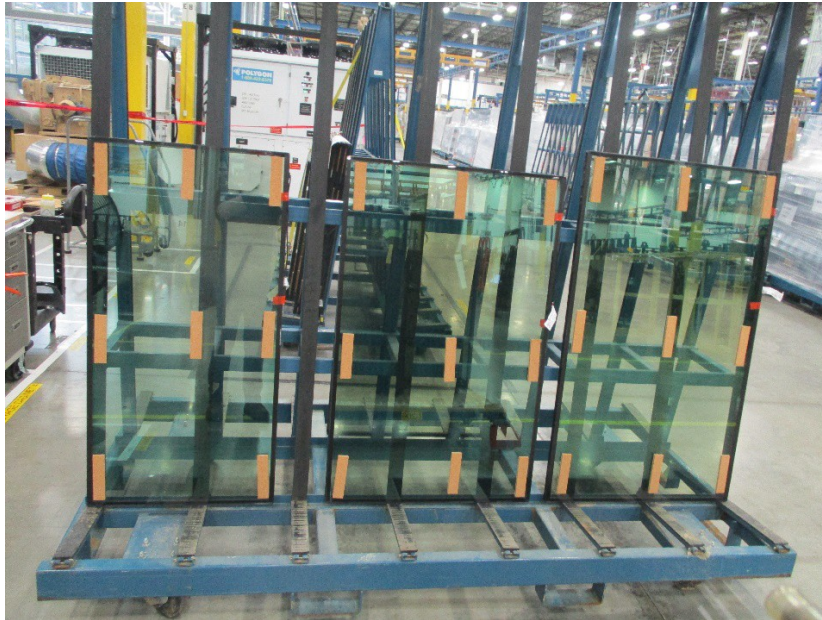
Figure 15: Cork pads are placed between each of the units when loading.
