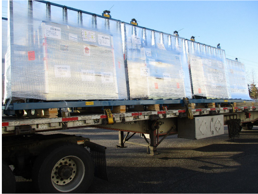
Figure 21: Frames are strapped underneath as required prior to leaving the facility. Straps or chains are acceptable. (NO STRAPPING OVER TOP.)
