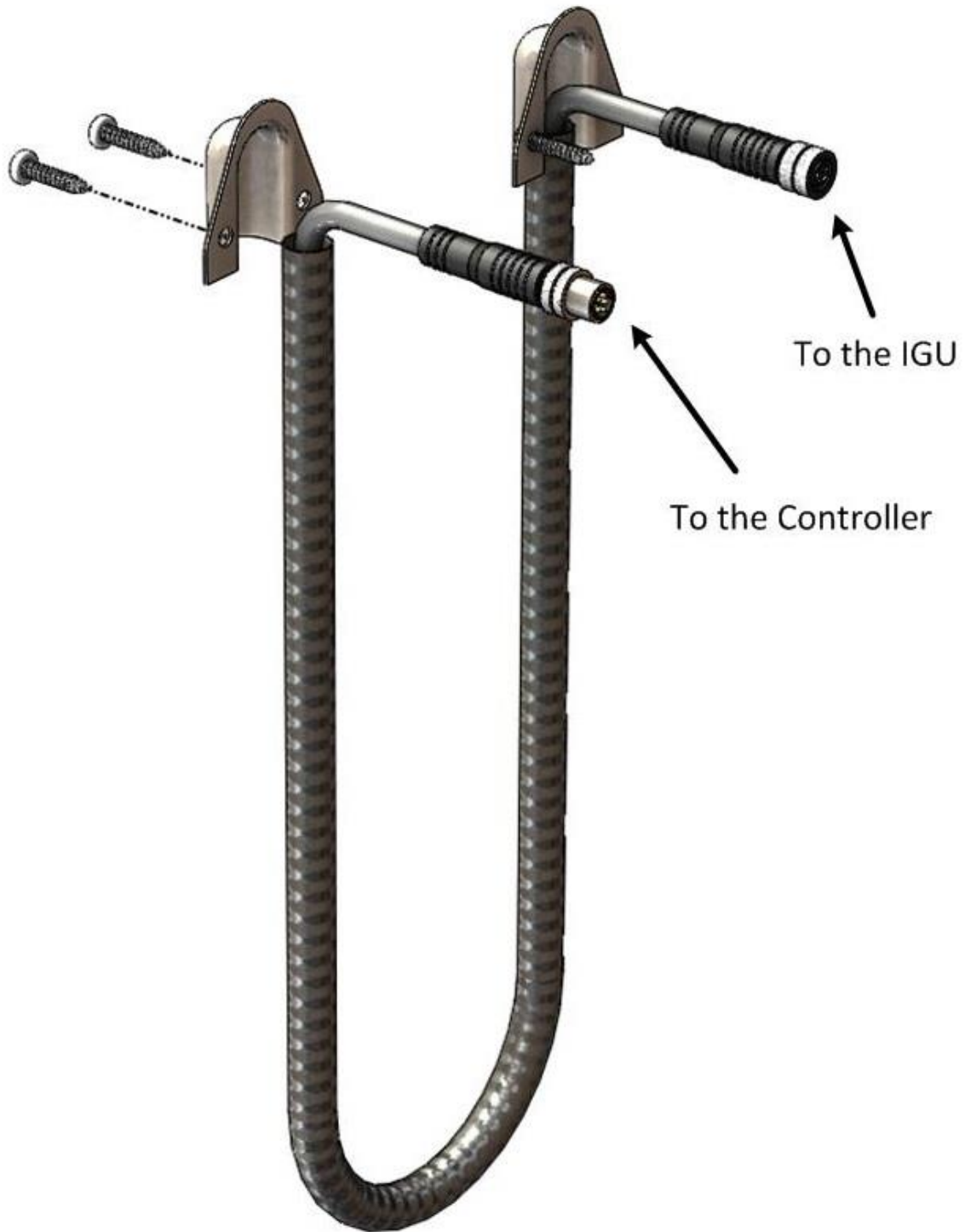
Figure 4 - An alternate design Door Loop Assembly - View model number VP - DL - SS - 000
