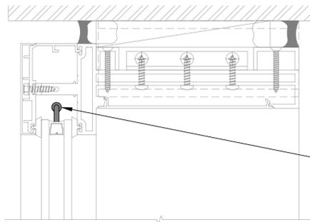
IGU CABLE CONNECTION TO IGU SWC IN GLAZING POCKET. RUN CABLE TO VERTICAL IN GLAZING POCKET
