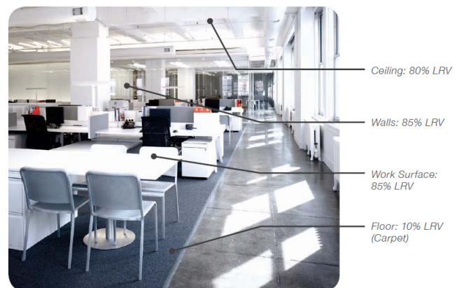
This high performance interior is designed to limit direct sun only to the transition/circulation space. Note the LRVs of the ceiling, walls and work surfaces - which help achieve maximum energy efficiency.
